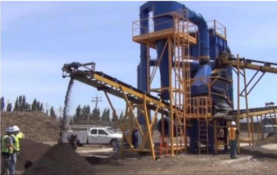
Densimetric separator at compost site in Gilroy, good at removing glass, rocks, rigid plastic.
