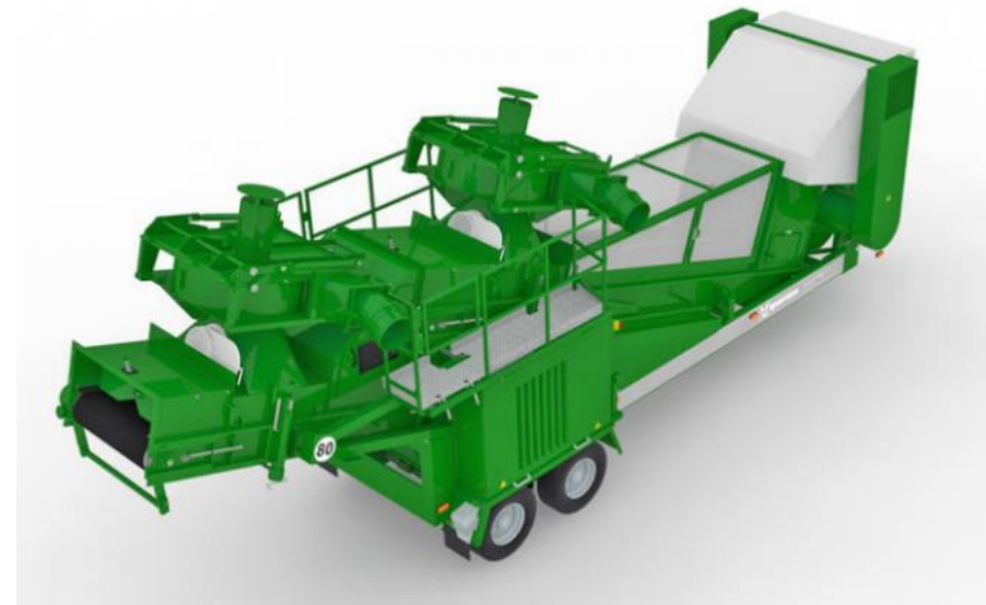
"Hurricane" air lift separator works well on film plastics.
